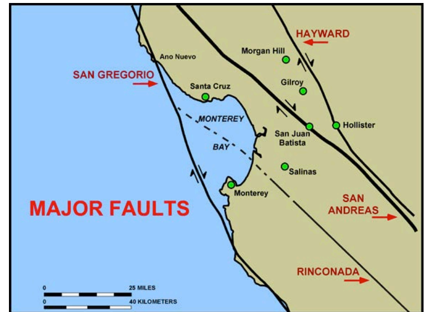
Figure 32. Major faults in the Monterey Bay area. Their displacements reflect the interaction of the great crustal plates that created them.
